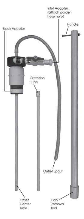
NOTE: 6mm (1/4 inch) diameter max. particle size.
